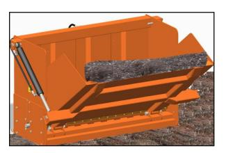
Note: When loading the chemical broadcaster ensure the manure is loaded evenly in the hopper.
