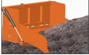
Lift the tailgate to the upper to keep the compost in the centre of the hopper
